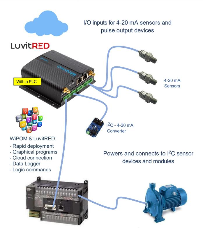
Manage, upgrade and access PLC's and sensors remotely.
